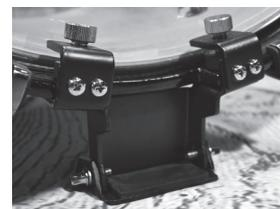
MBL909 "lift" goes at the hoop cut-out location. This gives clearance for the pedal chain and allows for the beater to hit at 12:00 (vertical) contact.
